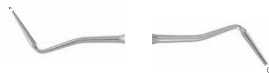
Mortenson #2 The blades are extra long and tapered with non-serrated tips. The tapered blades have the following diameters: 1.9-1.1 mm and 1.6-0.5 mm.
