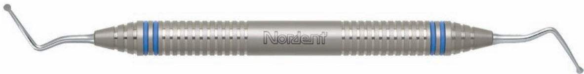
#33L The spoon shape blade diameter is 2.0 mm. The curved terminal shank is 15 mm long and set at a 60° angle to the center line of the handle. Handle Selection: CEEC33L (shown) REEC33L EC33L
