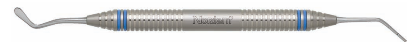
Glick #1 The plugger has markings at 5 mm and 10 mm. It can be used to condense gutta-percha and can be heated to sever excess gutta-percha. The paddle is used to place materials.
